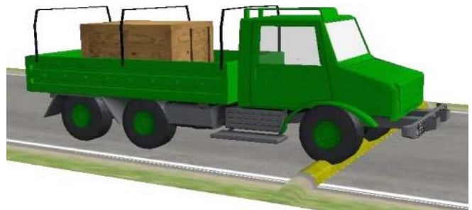
Figure 4: Simulation of half-round single curb strike.
